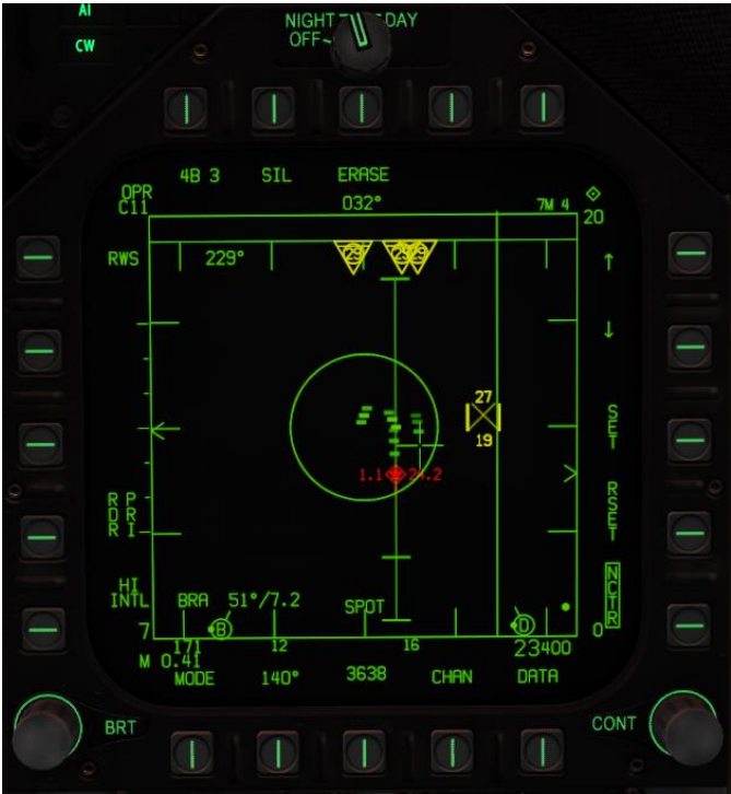
Figure 85. SPOT Sub-Mode
