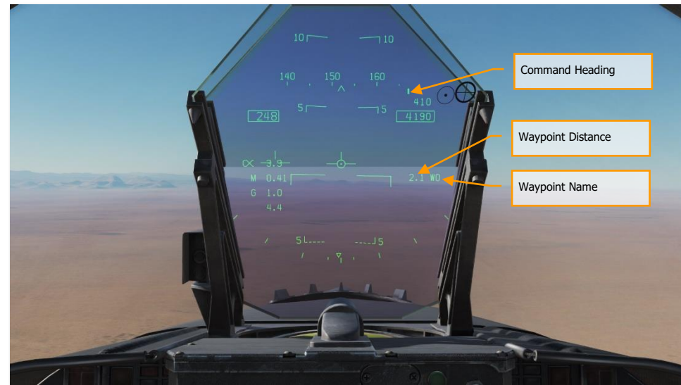
Figure 43. Waypoint Steering on HUD
