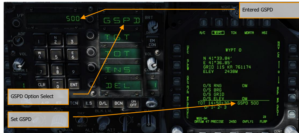
Figure 47. Ground Speed Data Entry
