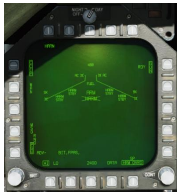
Figure 207. "HARM" Label Crossed Out.
