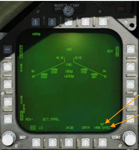
Figure 205. HRM OVRD inactive, Pullback mode active
