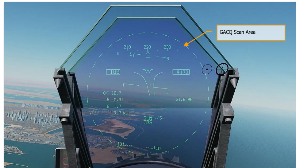
Figure 137. A/A GUNS Auto Acquisition Area
