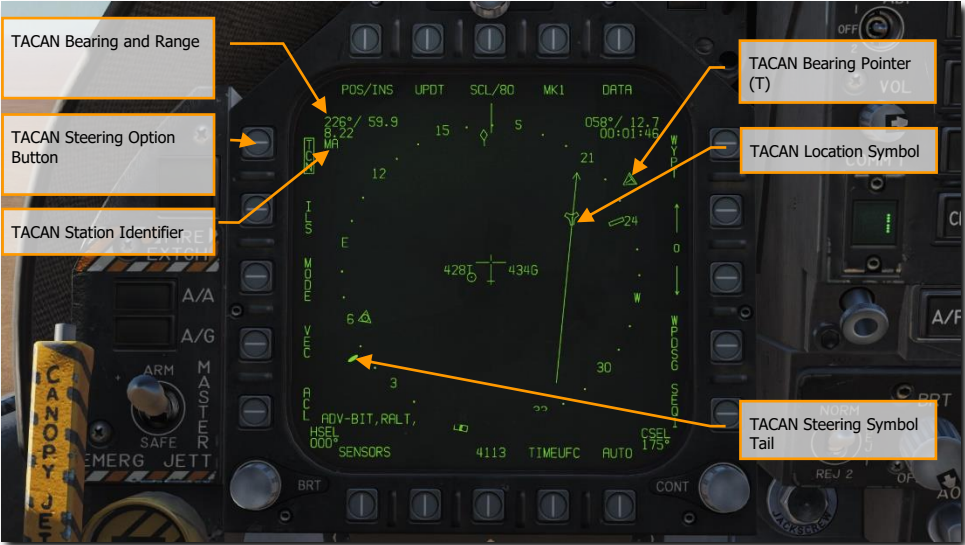
Figure 62. TACAN Steering on HSI
