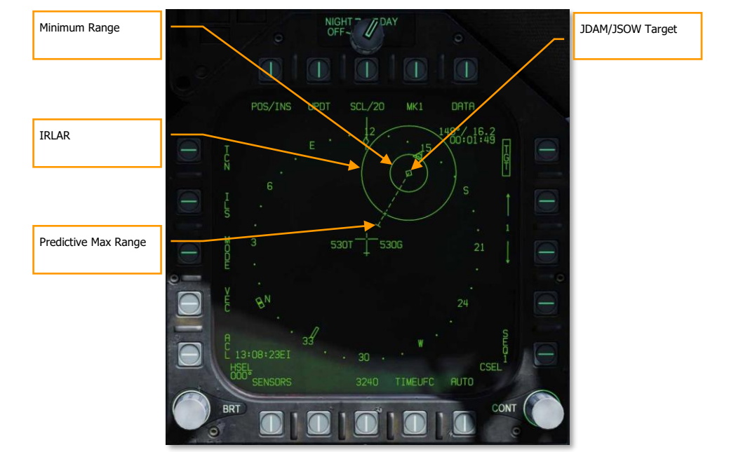
Figure 185. GPS Weapon HSI Format
