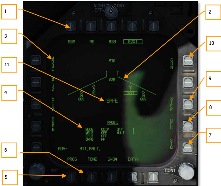
Figure 160. A/G Conventional Bombing SMS Page
