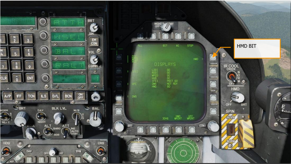
Figure 125. HMD Built in Test (BIT)
