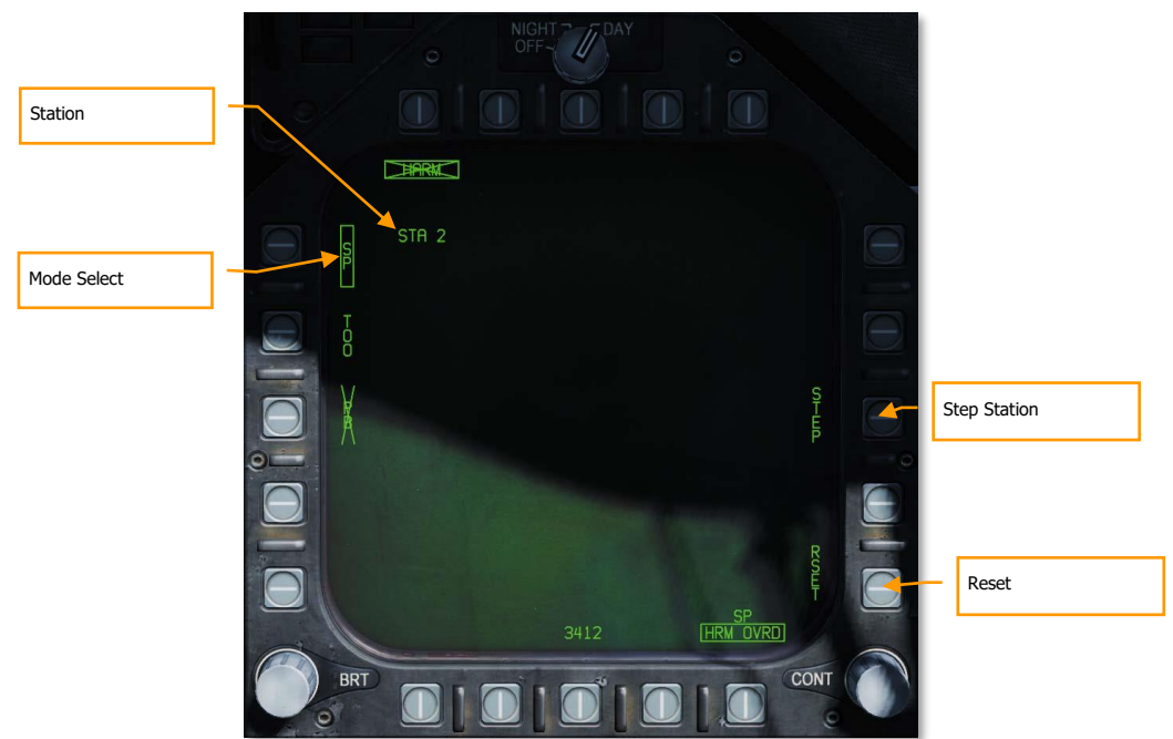
Figure 203. HARM SP SMS Format
