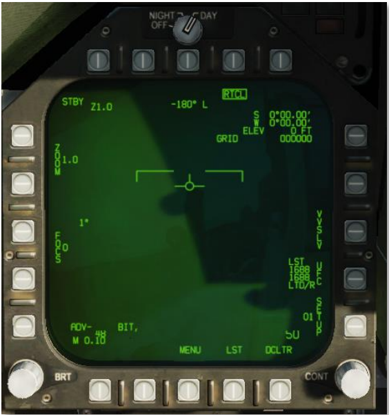
Figure 105. ATFLIR format in STBY mode.
