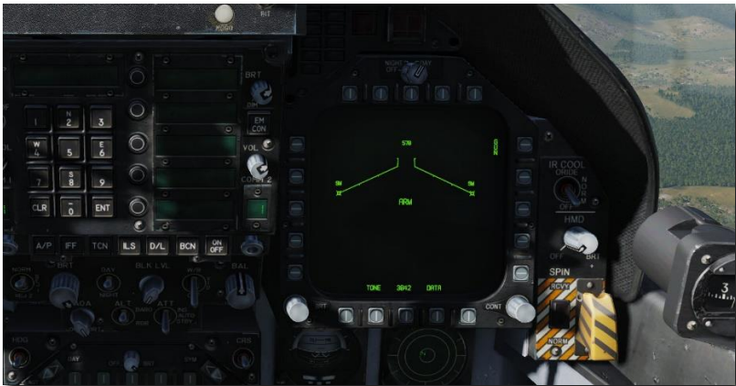
Figure 35. Stores Management System (SMS) Page
