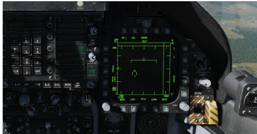
Figure 37. Attack Radar Page
