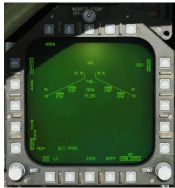
Figure 208. "PLBK" label displayed when Pullback is inhibited.
