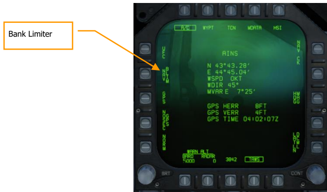
Figure 72. Coupled Autopilot Controls on HSI A/C Page
