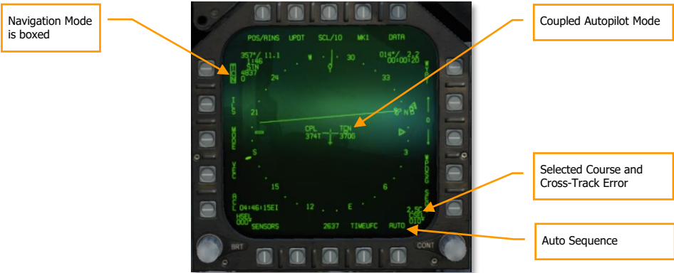
Figure 71. Coupled Autopilot Controls on HSI
