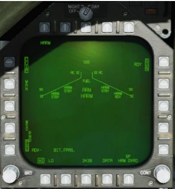
Figure 206. "HARM" displayed on Stores page and HUD.
