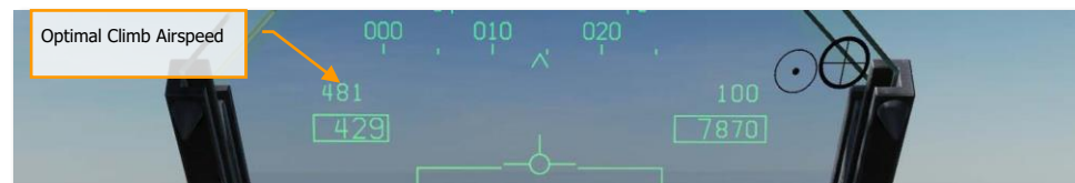
Figure 32. Optimal Climb Selection
