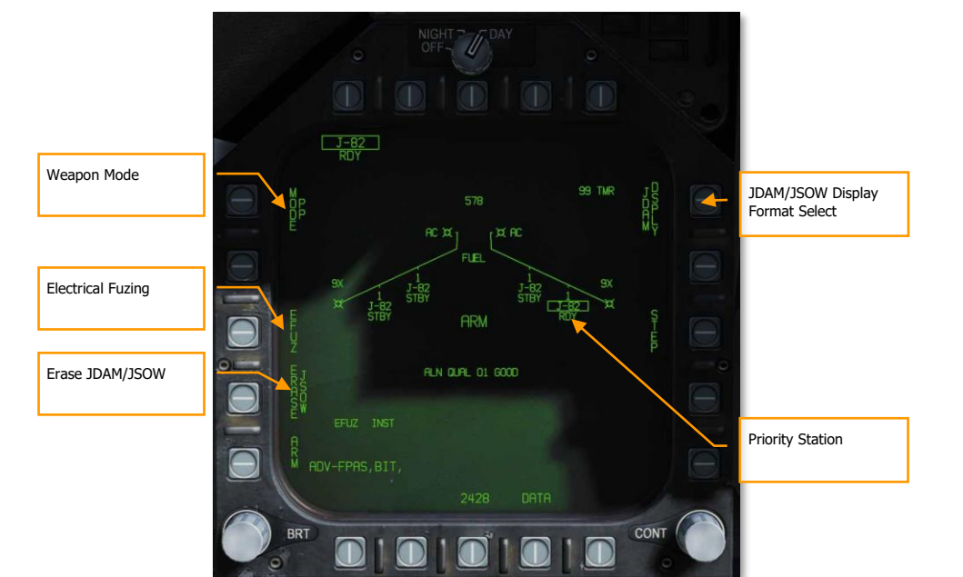
Figure 181. GPS Weapon SMS Format
