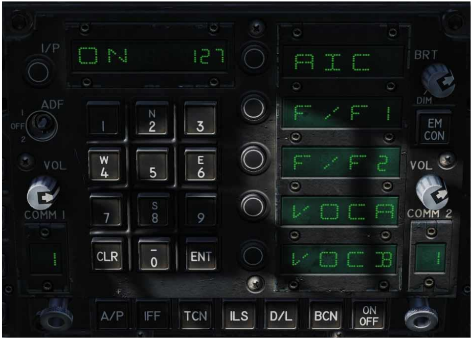
Figure 97. Datalink (D/L) UFC
