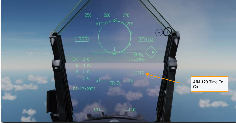
Figure 157. AIM-120 Radar Tracking, Post Launch HUD
