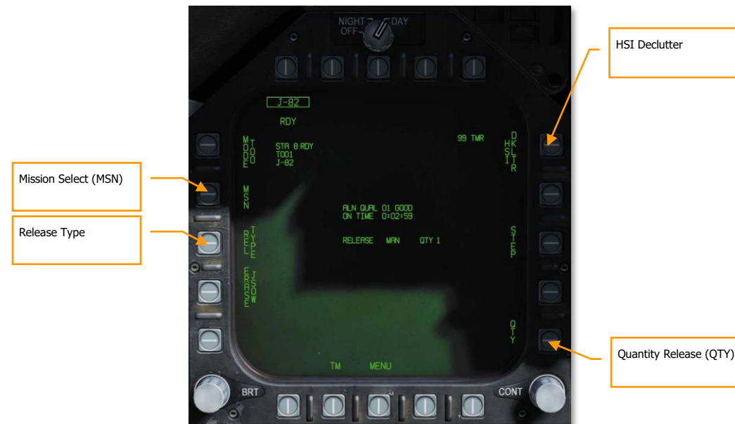
Figure 182. GPS Weapon SMS Format
