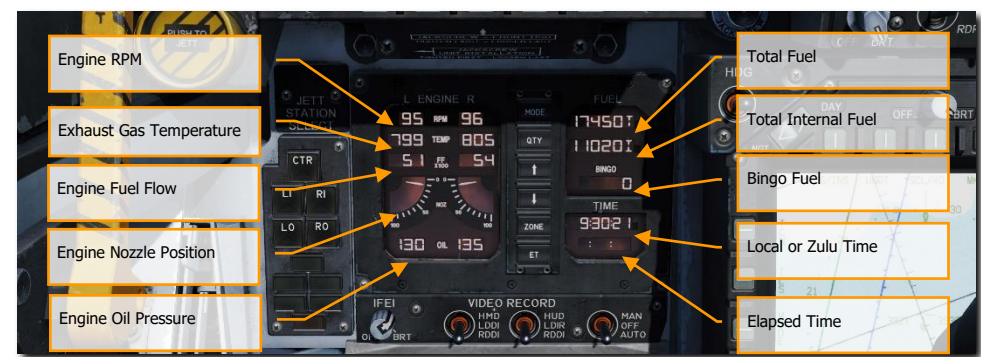
Figure 4. Integrated Fuel / Engine Indicator (IFEI)
