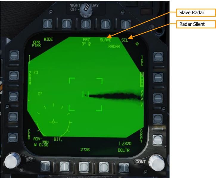
Figure 124. FLIR Air-to-Air Format (Tracking)
