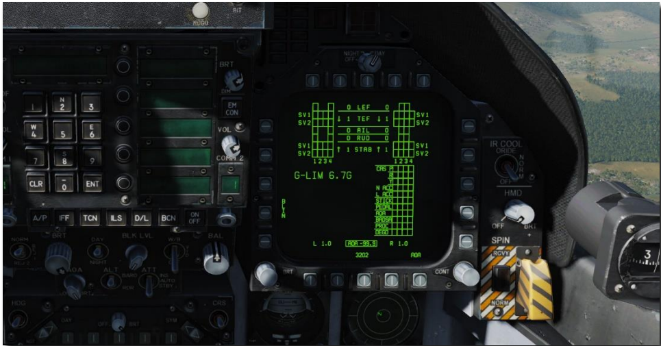
Figure 27. Flight Control System (FCS) Page
