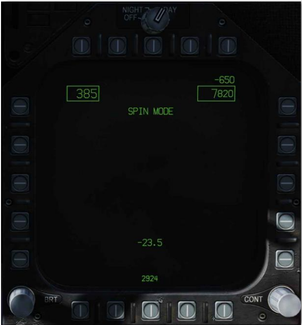
Figure 13. Spin Recovery Display
