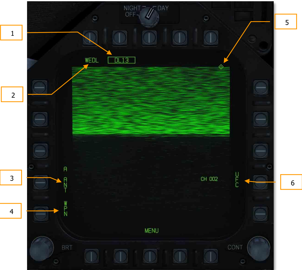
Figure 227. Datalink Only Format
