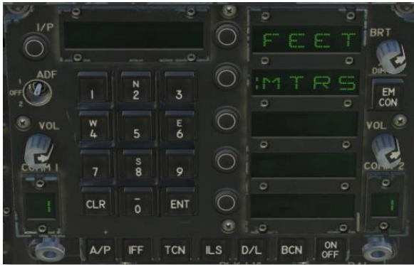
Figure 54. Offset Aimpoint Elevation Menu
