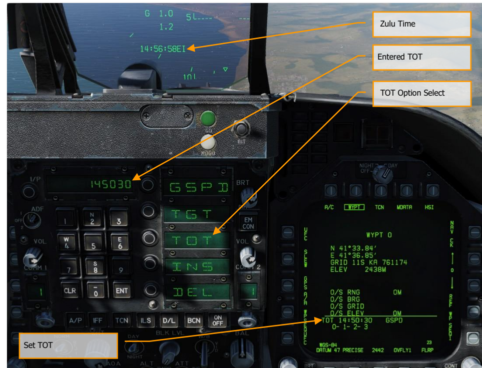
Figure 46. Time on Target Data Entry
