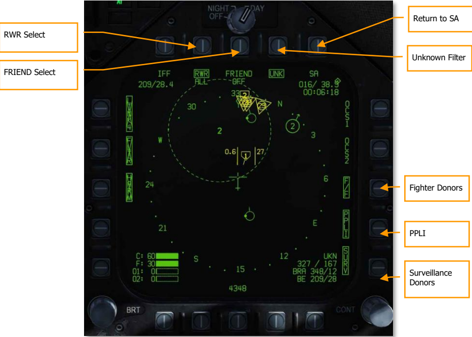
Figure 99. SA Page Sensors Sub-Level
