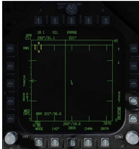
Figure 79. Bullseye as Current Waypoint
