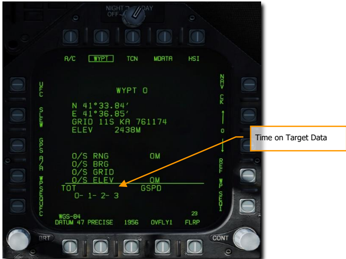
Figure 45. Time on Target Data Fields
