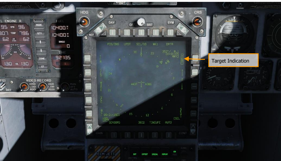
Figure 166. AUTO Bombing, Waypoint Designated as Target (TGT)
