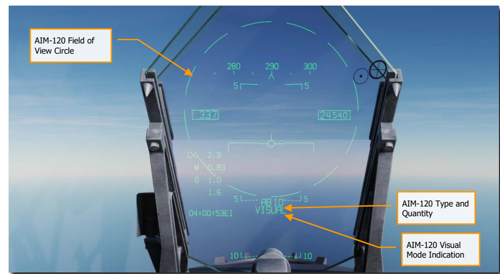
Figure 153. AIM-120 HUD, No Target
