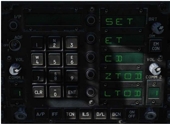
Figure 41. TIMEUFC Options on UFC
