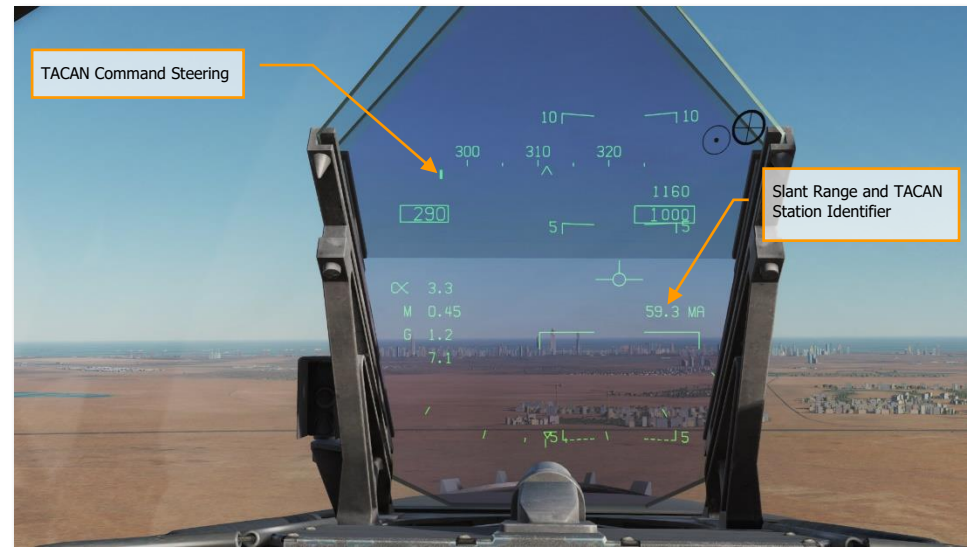
Figure 63. TACAN Steering on HUD
