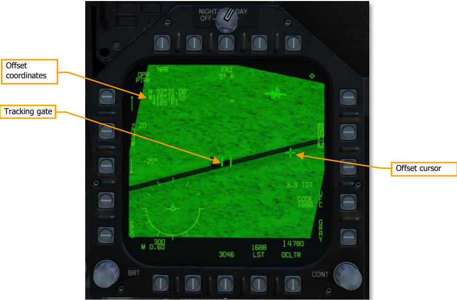
Figure 120. PTRK Mode with Offset Cursor
