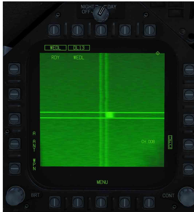
Figure 229. Combined Walleye and Datalink Format
