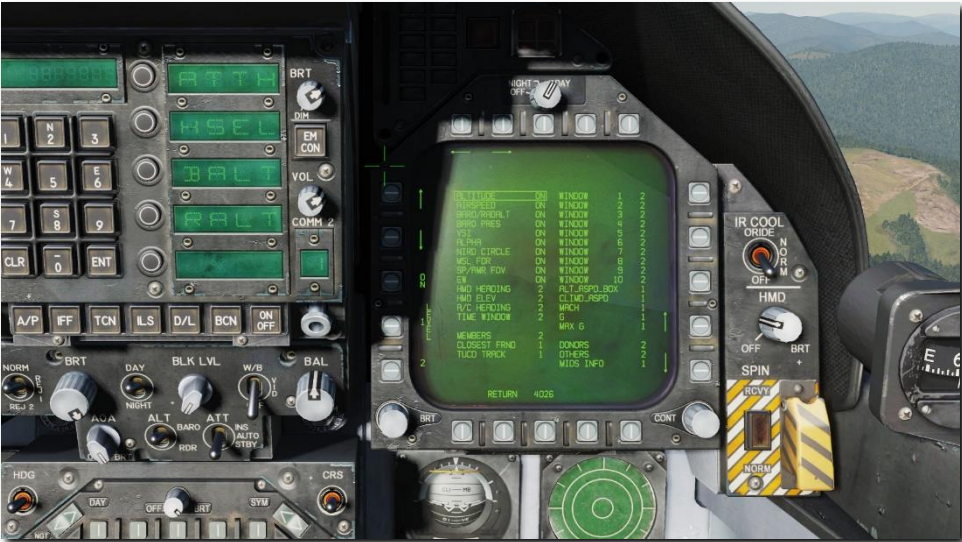
Figure 127. HMD Reject Setup Sub Level
