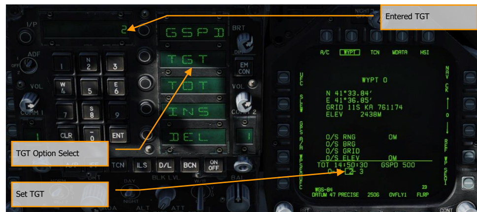
Figure 48. Target Data Entry
