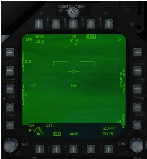
Figure 116. ATFLIR Air-to-Air mode, post-designate
