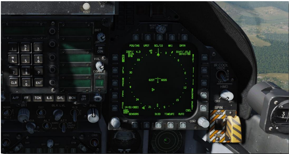
Figure 30. Horizontal Situation Indicator (HSI) Page
