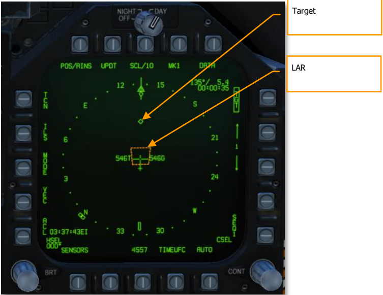
Figure 178. HSI Format, Paveway III Attack
