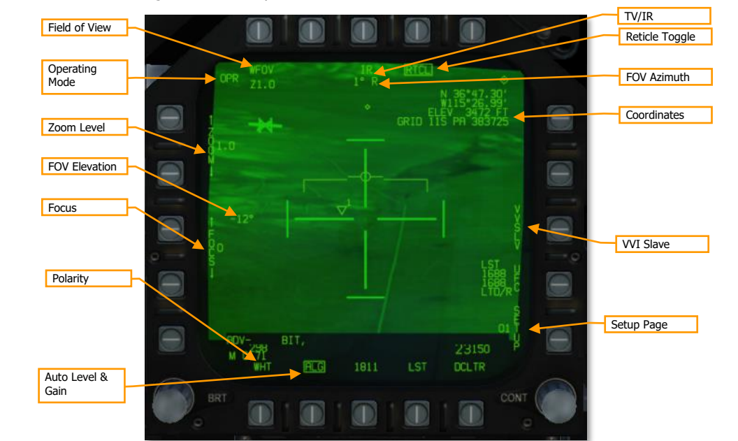
Figure 106. ATFLIR format in OPR mode (controls).
