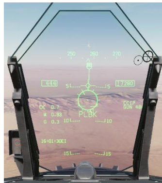
Figure 208. "PLBK" label displayed when Pullback is inhibited.
