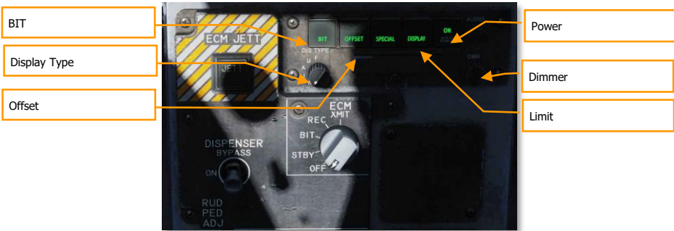
Figure 234. Control Indicator Panel
