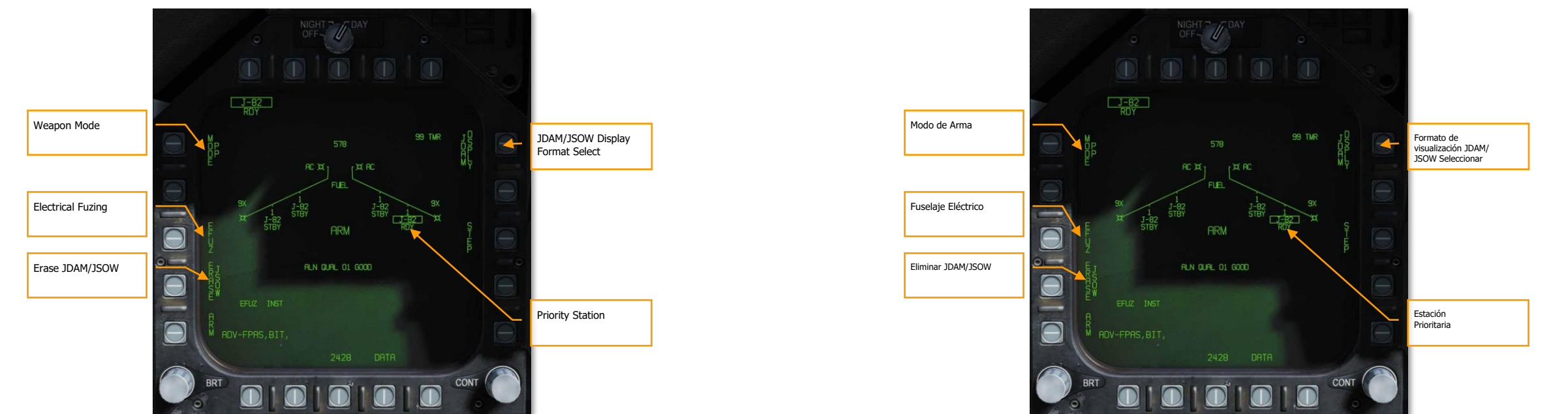
Figure 181. GPS Weapon SMS Format
