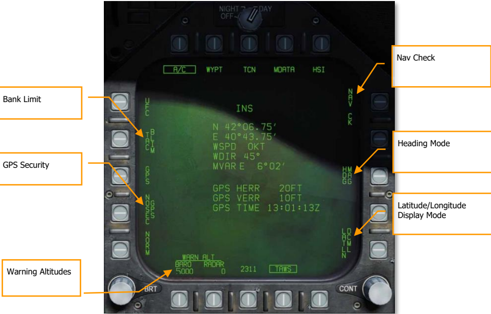
Figure 64. Aircraft HSI DATA Sublevel
