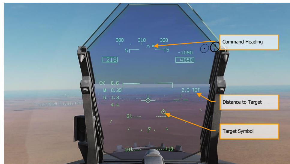
Figure 44. Waypoint as Target on HUD
